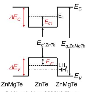
Fig. 1. Schematic band diagram of a ZnTe/ZnMgTe QW structure.
