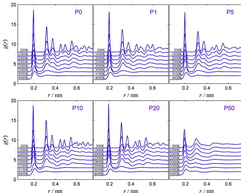
Fig. 1. RDF evolution at different pressures during quenching. ( $P_1 = 1$  GPa,  $P_5 = 5$  GPa,  $P_{10} = 10$  GPa,  $P_{20} = 20$  GPa, and  $P_{50} = 50$  GPa).
