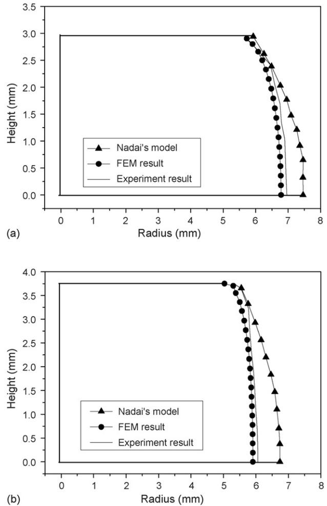
Fig. 1. Results of comparison data: (a) final shape after 42% reduction; (b) final shape after 35% reduction.
