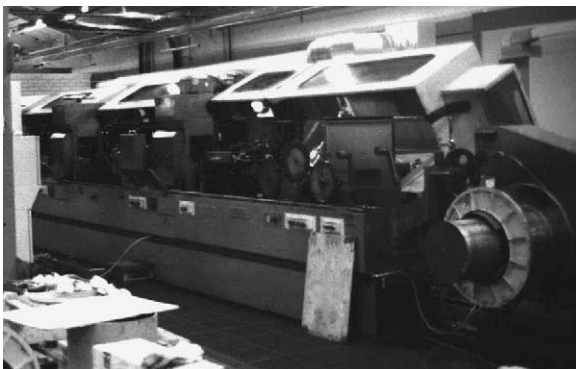
Fig. 2. The cold-rolling mill used for the present experiments. The final rolling pass is at the right end of the mill.
