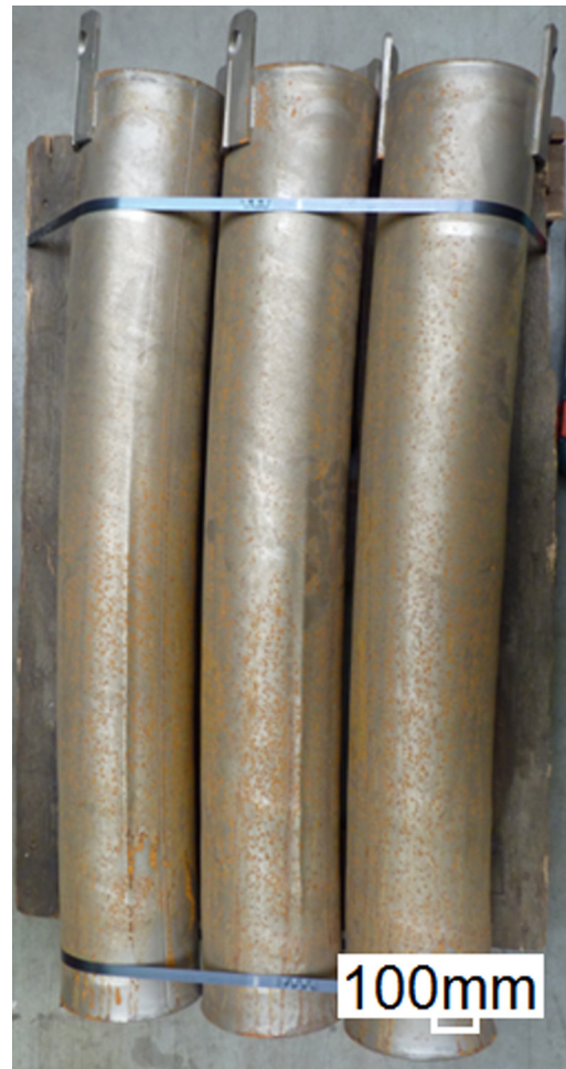
Fig. 1. Bended tubes after HIP (courtesy from Köppern Entwicklungs-GmbH).
