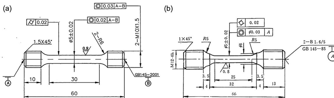
Fig. 1. Schematic diagram of standard tensile (a) and creep (b) specimen.
