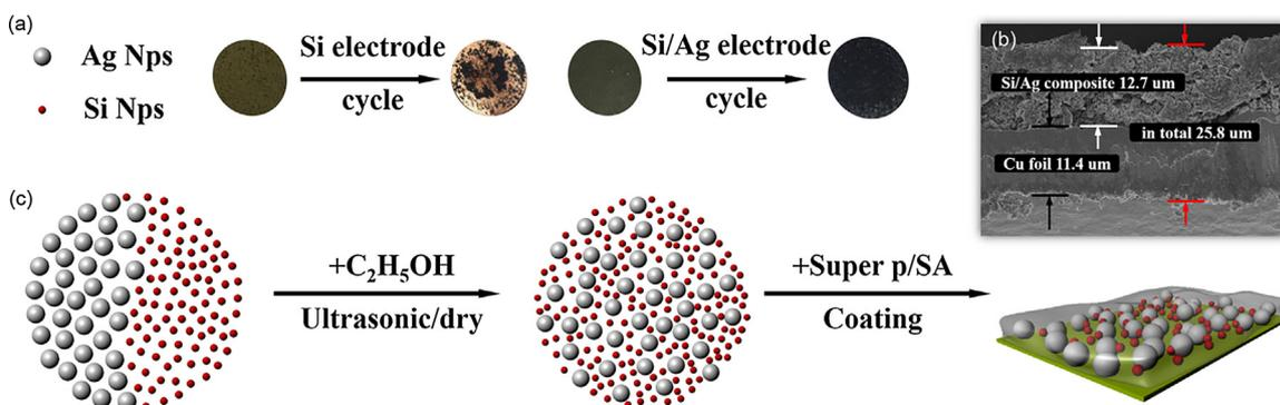
Fig. 1. Schematic of macroscopic visual change of electrodes after cycling test (a), cross-sectional view of newly prepared Si/Ag electrode with Si/Ag ratio of 1:1 (b) and fabrication process of Si/Ag electrode (c).
