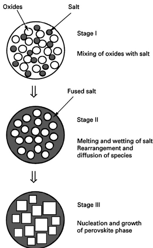
Fig. 1. Schematic illustration of the main processing stages of the MSS method for synthesis of perovskite oxide powders.
