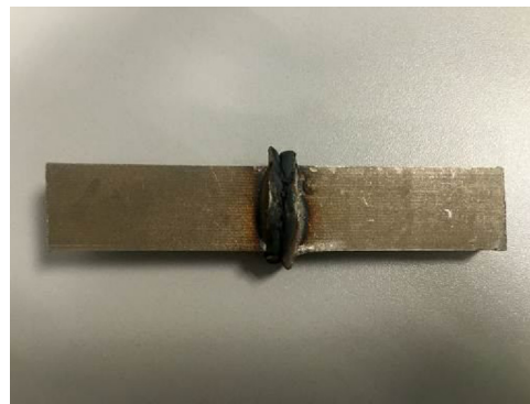
Fig. 2. Appearance of the welded joint.
