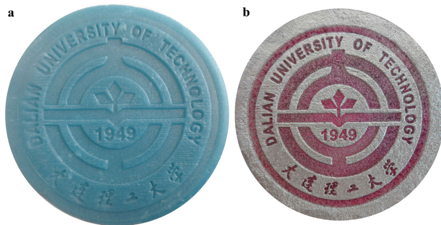
Fig. 1. Dalian University of Technology emblems formed by hand stamping on (a) plain plasticine and (b) metallic plasticine (GaInSnCdZn 2 alloy) at 30–40 °C, respectively.
