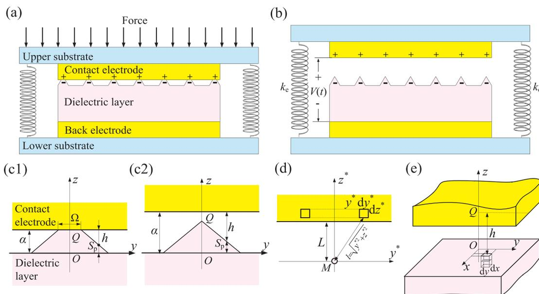
Fig. 1. Schematic diagrams of (a) contact and (b) separation states of a spring-based TENG, (c) the adhesive contact and separation between the electrode and textured layer, (d) adhesive contact between the electrode and a molecule in the dielectric layer, (e) adhesive contact between the electrode and a micro-element body on the textured dielectric layer with textures omitted.
