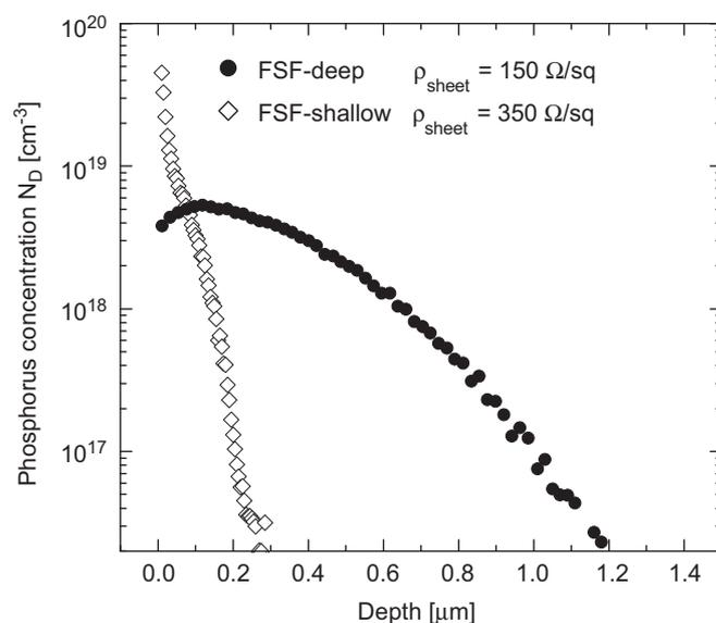
Fig. 2. Secondary ion mass spectroscopy (SIMS) profiles of the studied phosphorus dopant profiles measured after all high temperature processing steps. Sheet resistance of both diffusion profiles is shown in the graph.
