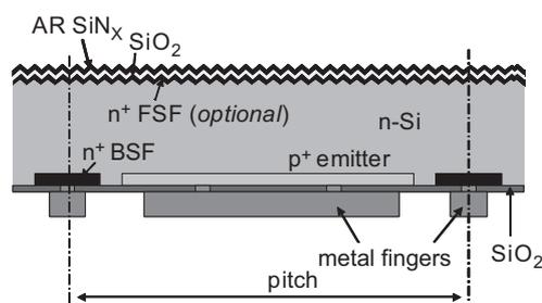
Fig. 3. Schematic cross-section of the n-type high-efficiency back-contact back-junction silicon solar cell investigated in this work. Note that sketch is not to scale.
