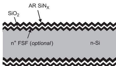
Fig. 1. Textured symmetrical structures used for the lifetime measurements and for the determination of the surface recombination current density.
