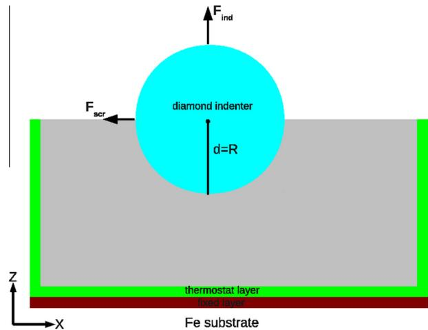
**Fig. 1.** Setup of the scratching system. The indentation depth  $d$  is equal the radius of the indenter  $R$ . The normal force  $F_{ind}$  and scratching force  $F_{scr}$  are shown. The substrate has thermostatting and rigid zones at its boundaries.
