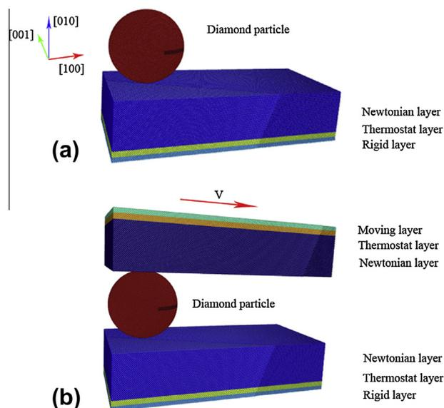
Fig. 1. The atomic model of the (a) two-body abrasion and (b) three-body abrasion.
