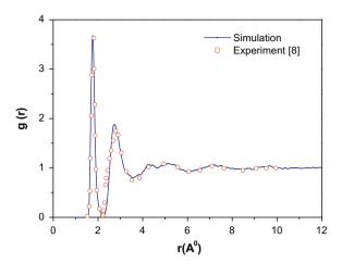
Fig. 2. The total PRDFs of a-Al $_2O_3$  at the density of 3.13 g cm $^{-3}$  and experimental data [8].
