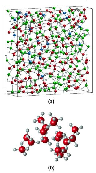
**Fig. 1.** (a) The structure of the central region (red:  $Al_4$ , green:  $Al_5$  and blue:  $Al_6$ ) and (b) a poly-PTE in the sample M3 (large and small spheres represent Al and O, respectively). (For interpretation of the references to color in this figure legend, the reader is referred to the web version of this article.)
