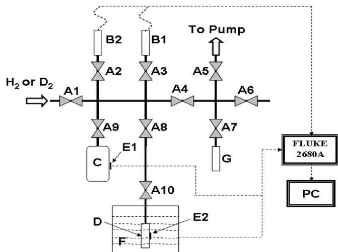
**Fig. 1.** Experimental system of the pressure-composition isotherm measurements. A1 ~ A10 — valves; B1 — 25 bar manometer; B2 — 0.25 bar manometer; C — standard pressure vessel; D — palladium bed; E1-E2 — Pt100; F — thermostat; G — vacuum gauge.
