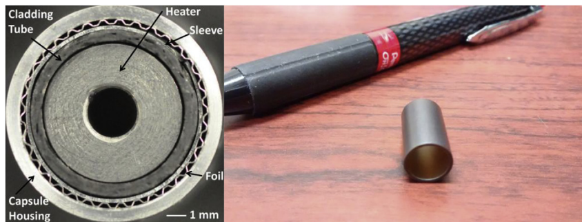
Fig. 1. Cross-section of assembled rabbit capsule (left) [11] and a CVD SiC tubular specimen (right).
