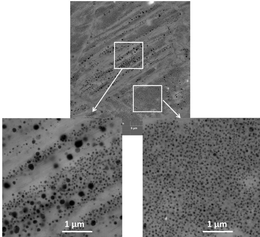
**Fig. 1.** A SEM-BSE image obtained by using 30 keV electron analysis beam and from Russian EK-164 fuel cladding irradiated to 82 dpa at 515 °C. These micrographs were supplied by Vladimir Pashtukov of the Institute of Nuclear Materials [25].
