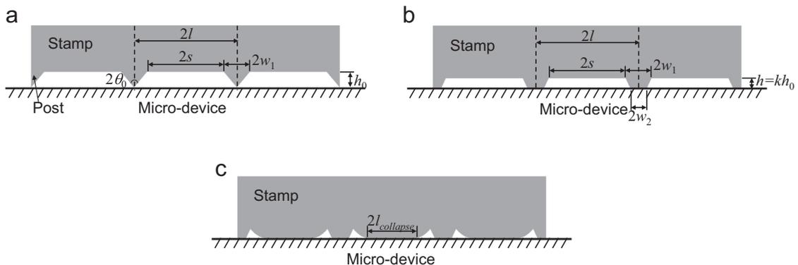
**Fig. 1.** Schematics of the microstructured stamp in contact with the flat surface of the micro-device. (a) The permanent configuration of the stamp with triangular posts in the absence of roof collapse; (b) the temporary configuration of the stamp with trapezoidal posts in the absence of roof collapse; and (c) the temporary configuration of the stamp with trapezoidal posts in the mode of roof collapse.
