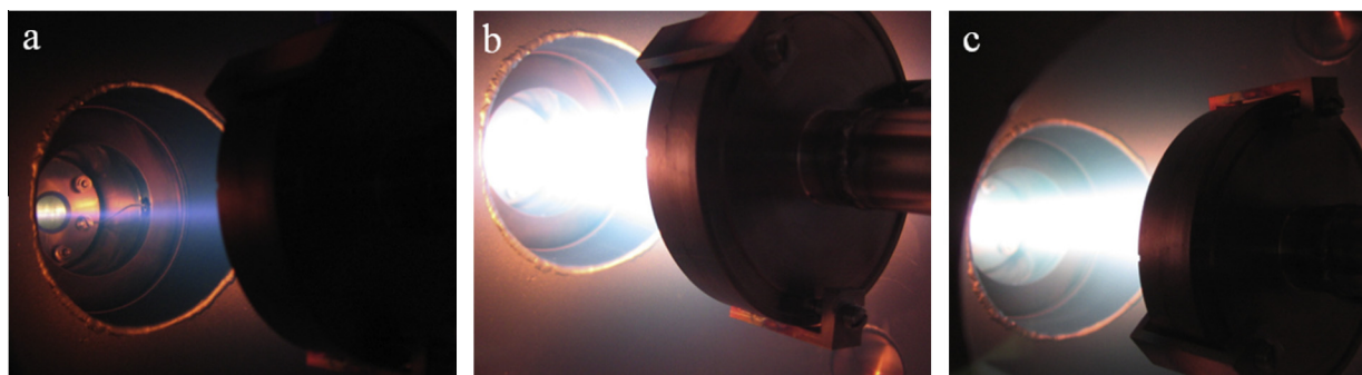
Fig. 2. Picture of main regimes of KTM PBF with Ar feeding: (a) mode I – pressure less than 0.1 Pa, accelerating voltage 6.0 kV, electron beam current 0.10 A, (b) diffusive BPD mode II 0.12 Pa, 6.0 kV, 0.11 A, (c) mode III with stabilized radial drift 0.2 Pa, 6.0 kV, 0.12 A.
