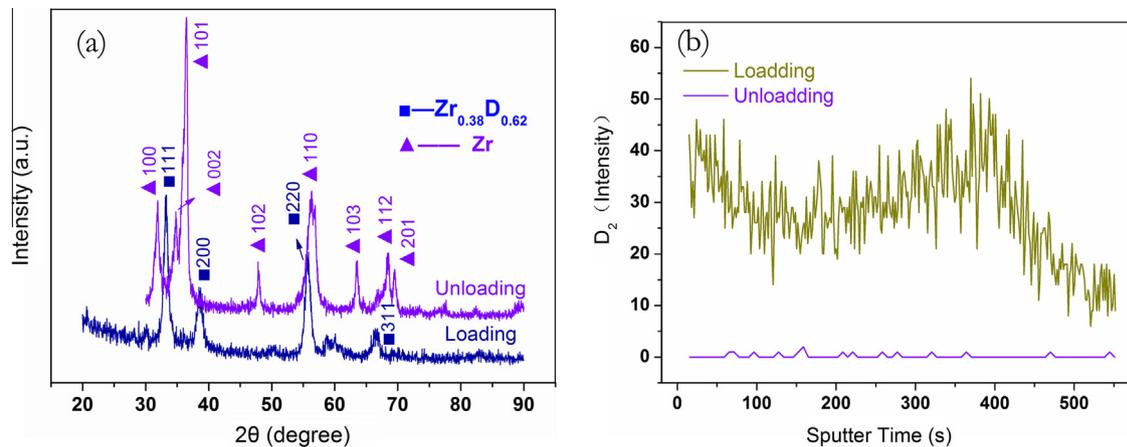
Fig. 1. XRD patterns of the films unloading and loading deuterium (a) and the SIMS results of Zr and deuteration elements by using the flux of oxygen (b).
