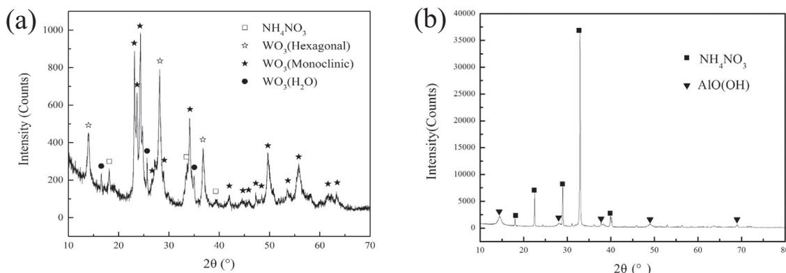
Fig. 2. XRD patterns of the hydrothermal products (a) I and (b) II.
