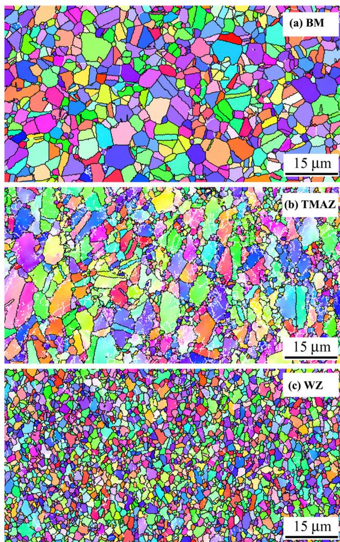
Fig. 2. Typical grain structure of (a) BM, (b) TMAZ and (c) WZ.
