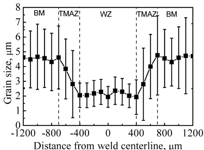
Fig. 1. Distribution of average grain size across WZ along tube wall edge.
