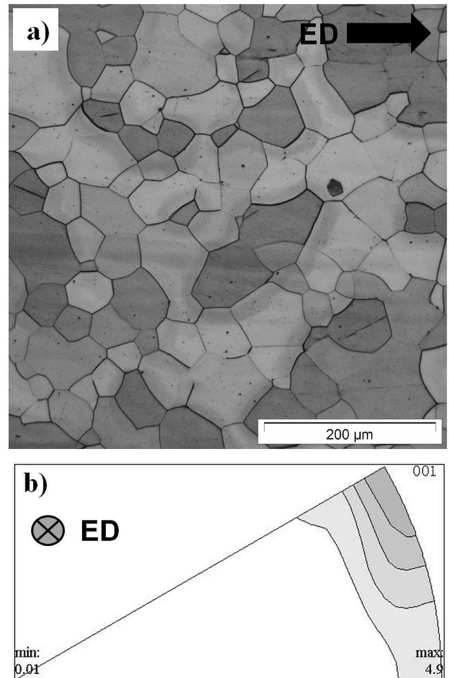
Fig. 1. Microstructure (light microscopy) (a) and texture (b) of extruded Mg–1Zn alloy in initial state.
