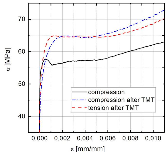
Fig. 2. Stress vs. strain dependences for compression tests of the Mg–1Zn alloy in as-extruded state and after thermo-mechanical treatment (TMT): pre-compression up to 75 MPa (or 2.7% of strain) and annealed at 200 °C for 8 h.
