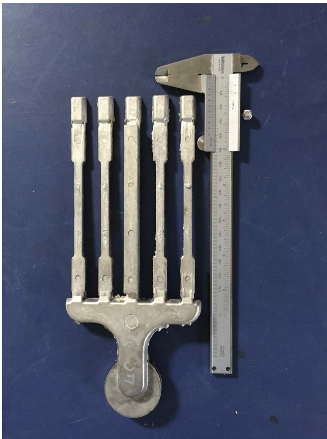
Fig. 1. Macrograph of experimental alloy cast.
