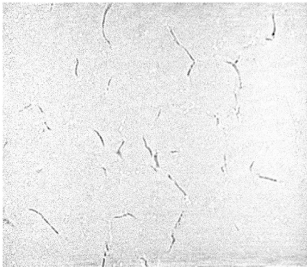
Fig. 3. Computed cross section of absorption contrast showing dark hydride phase.
