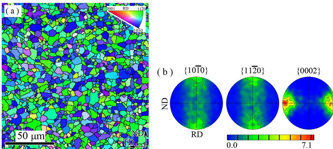
Fig. 1. Starting (a) microstructure and (b) texture of Zr-4 alloy.
