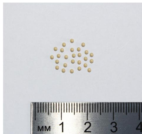
Fig. 1. The photo of baddeleyite origin beads sintered at a temperature of 1350 °C.
