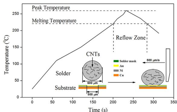
**Fig. 1.** Schematic drawing of reflow profile applied for solder ball and solder joint fabrication.
