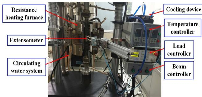
Fig. 1. Experimental setup for the creep-fatigue experiments.
