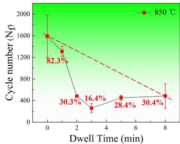
Fig. 3. Relationship between the dwell time and fatigue life (number of cycles to fracture) for the directionally solidified Ni-based superalloy DZ445 samples.
