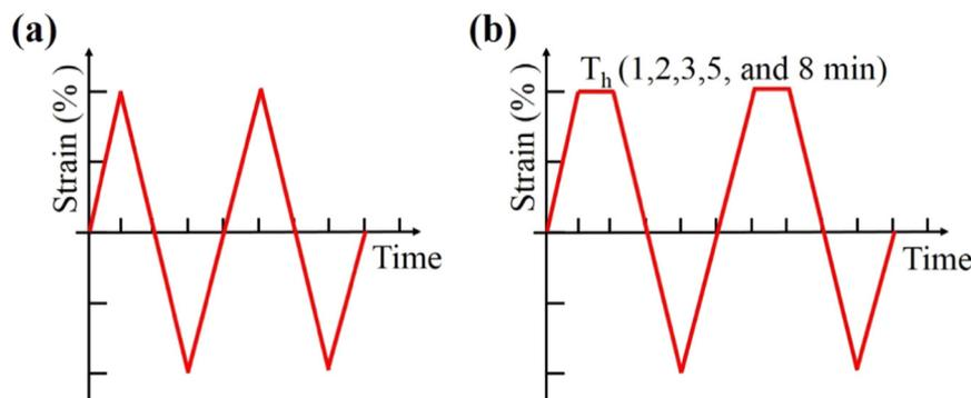
Fig. 2. Waveforms of the total strain-controlled creep-fatigue tests (a) without dwell time (b) with dwell time.
