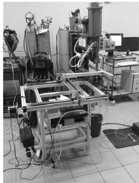
Fig. 1. An automated stand for spot welding according to PN-EN ISO 8166:2007 standard.
