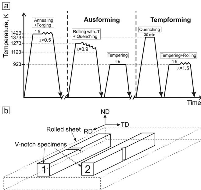
Fig. 1. Schematic diagrams illustrating the routes of thermo-mechanical processing (a) and the specimen orientations for impact tests (b).
