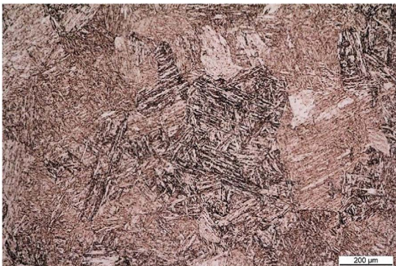
Fig. 1. As-received microstructure of the investigated 10%Cr steel (optical microscopy image, etchant: warm picric acid).
