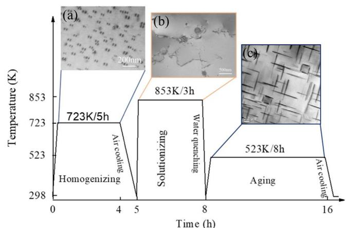
Fig. 1. A schematic diagram illustrating the heat treatments and involved microstructural evolution.
