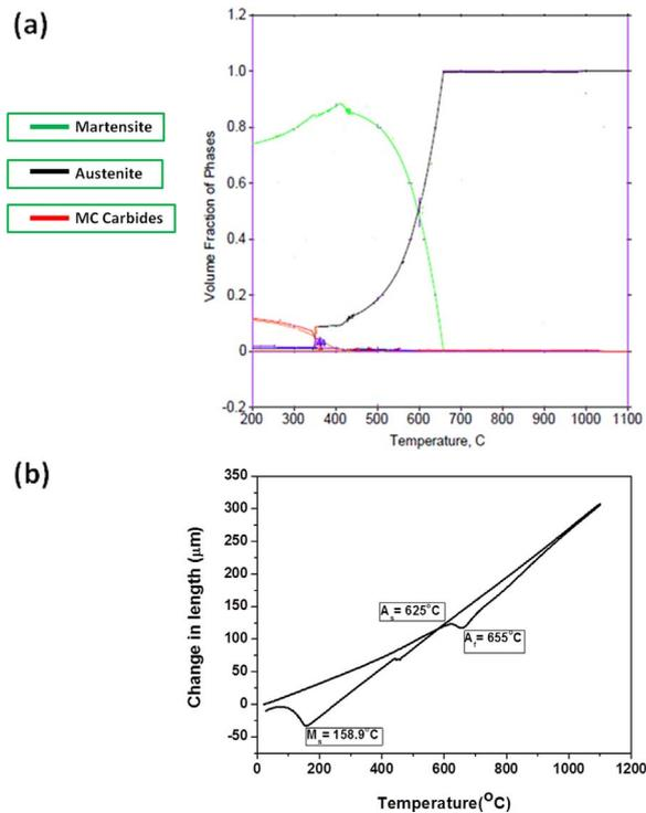
**Fig. 1.** (a): Phase variation chart for 12Cr-10Ni steel calculated by Thermo-Cal™ software in the temperature range of 200–1100 °C. (b): Results of dilatometry for 12Cr-10Ni steel from room temperature to 1100 °C at a heating and cooling rate of 5 °C/min.
