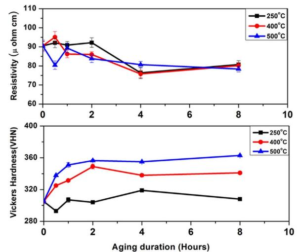
**Fig. 3.** Variation of electrical resistivity and Vickers hardness with ageing time. These are shown for samples solution treated at 1000 °C and then subjected to three different aging temperatures. Error bars represent standard deviations from multiple measurements.
