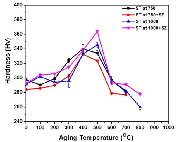
**Fig. 2.** Isochronal aging curves for 12Cr-10Ni samples solution treated at 750° and 1000 °C, and aged at various temperatures from 100 to 800 °C for 2 h. It is to be noted that both sets of solution treated samples are also subjected to sub-zero (SZ) treatment or quenching in liquid nitrogen. However, SZ samples do not show significant difference in ageing behaviour. Error bars represent standard deviations from multiple measurements.
