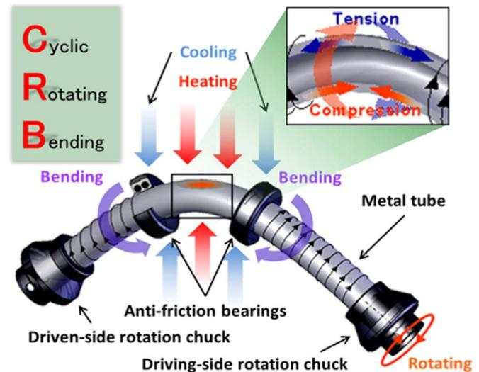
Fig. 1. Schematic illustration of the CRB process.
