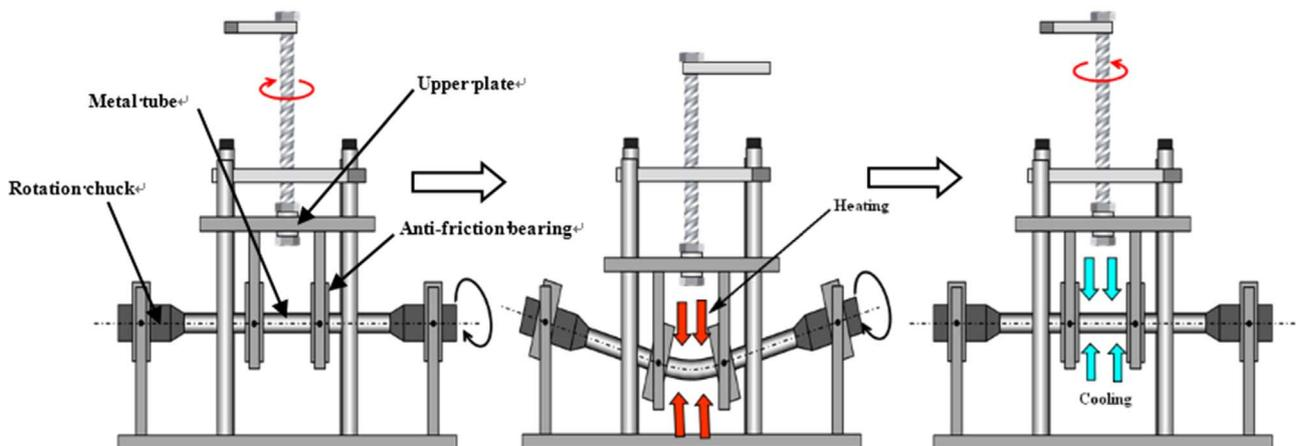
Fig. 2. Sketch map of implementation procedure of the CRB process.
