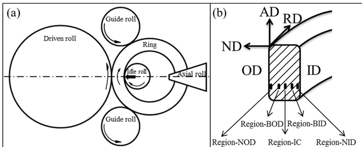
Fig. 1. (a) The schematic diagram of the hot radial-axial ring rolling. (b) The cross-section of the ring, definition of coordinate system and the investigated regions throughout the ring wall thickness.
