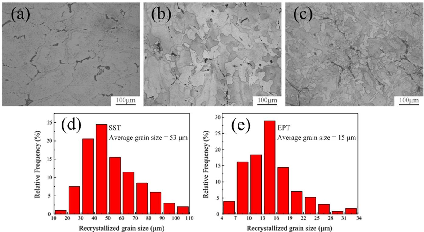
Fig. 1. Optical microstructures of (a) HR, (b) SST and (c) EPT samples, (d) and (e) recrystallized grain size distribution with different conditions.
