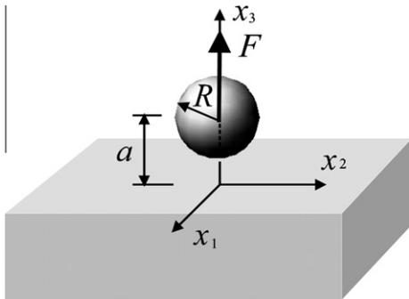
Fig. 1. A rigid nanoparticle located over an elastically incompressible semi-infinite substrate. An external force is applied to maintain the equilibrium.
