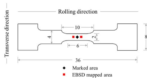
Fig. 1. Schematic of the specimen used for tensile test and EBSD (dimensions are in mm).
