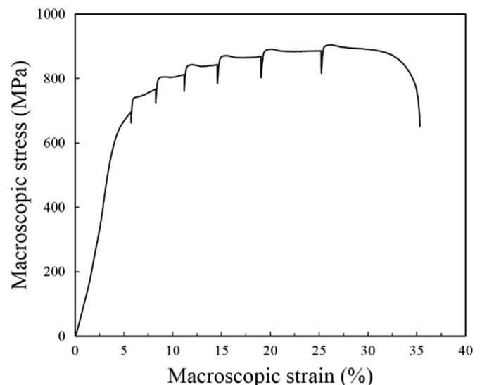
Fig. 2. Macroscopic stress–strain curves of the specimen recorded during the in-situ EBSD experiment.
