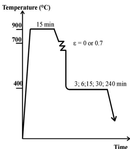
Fig. 1. Schematic representation of the thermomechanical processing route.
