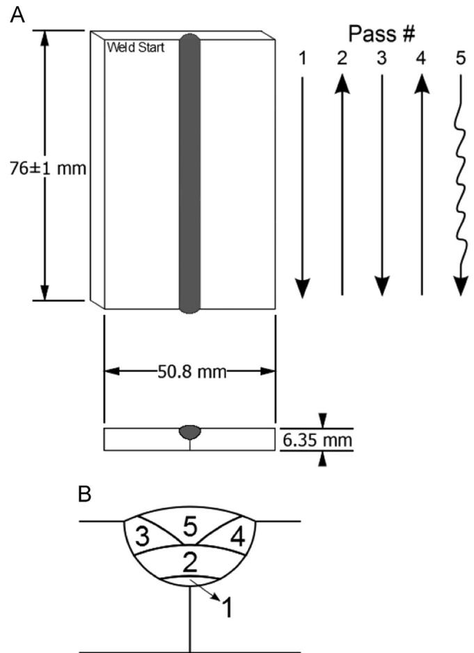
**Fig. 1.** A: Pass locations, directions, and weldment geometry used in the Co–AgCu TIG welds. Two cobalt samples sharing a single U-groove are joined by 5 passes in alternating directions. The final, oscillating pass is indicated by a wavy line. B: Approximate weld-bead locations. Dimensions are all  $\pm 0.08$  mm unless noted otherwise.
