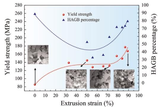
**Fig. 2.** YS vs. extrusion strain curve and percentage of HAGB vs. extrusion strain curve of CPAWs after cold drawing for different passes. TEM images of the CPAWs processed by cold drawing for 0, 2, 5 and 9 passes.
