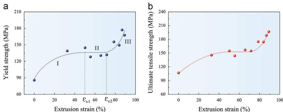
**Fig. 1.** Yield strength (a) and ultimate tensile strength (b) vs. extrusion strain curve for the cold-drawn CPAWs.
