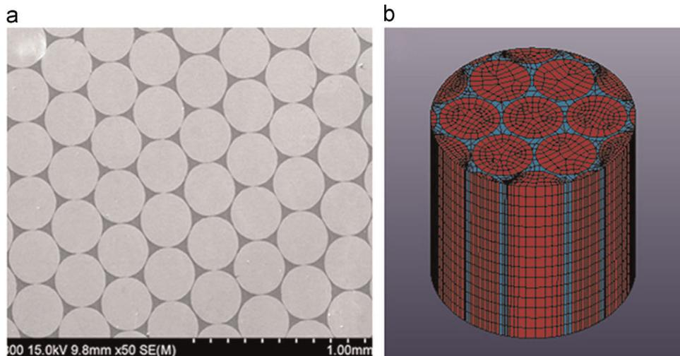
Fig. 1. SEM image of the composite with  $V_f$  of 83% (a) and the corresponding FEM model (b).
