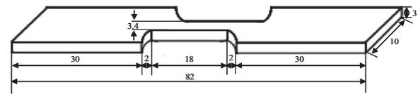
Fig. 1. Sketch of the flat sample (mm).
