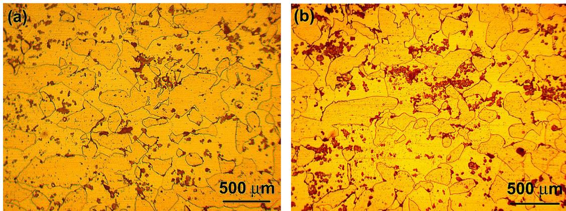
**Fig. 1.** Microstructure of the as-received materials used in this investigation: (a) CuZn39Pb2 and (b) CuZn39Pb3.
