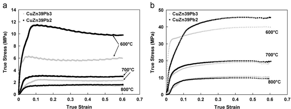
**Fig. 2.** Representative true stress–strain curves of the studied alloys at various temperatures and strain rates of (a) 0.001 s<sup>-1</sup> and (b) 1 s<sup>-1</sup>.
