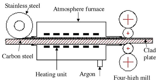
**Fig. 1.** Schematic of the hot roll bonding system.
