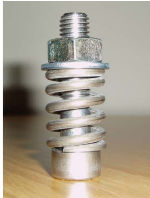
Fig. 1. The spring in the bolt assembly. The ends of the springs are flattened and tapered. The spring is subjected to a fixed compressive displacement \delta using a tightened nut and bolt.
