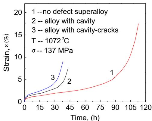
Fig. 1. Influence of the defects on creep properties of the alloy.
