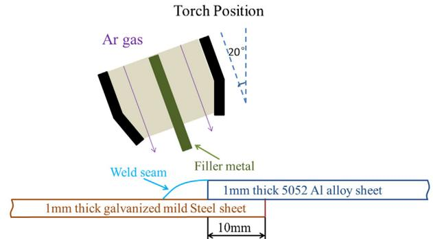
**Fig. 1.** Schematic diagram of the gas metal arc welding process.
